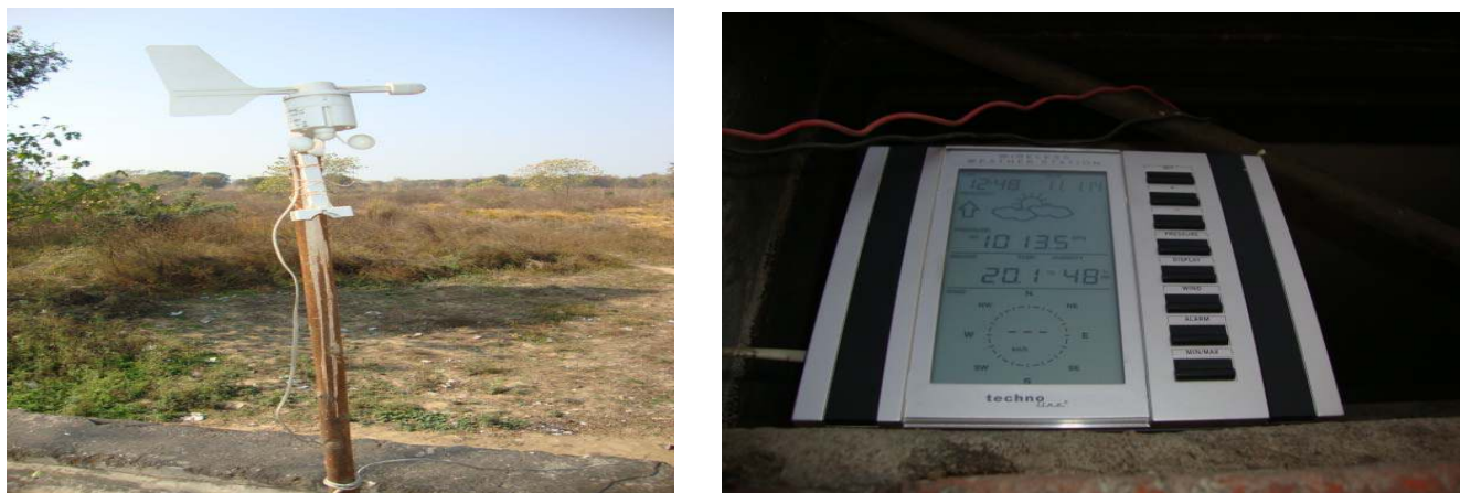
Pic. 5.2 Showing the wind monitoring station set up at the project site
